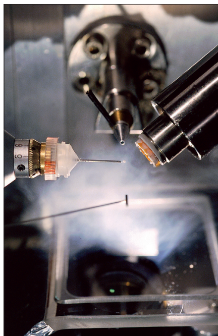
Tiny crystal: A crystalline protein sample ready for analysis in the X-ray beam at the ESRF.
