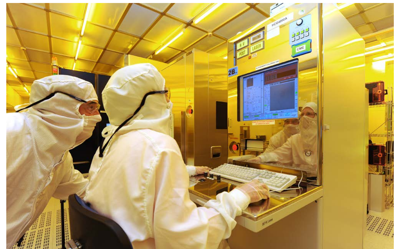
Clean room with Hitachi HCG4000 lithographic machine
