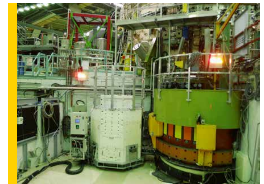
ILL LAGRANGE neutron spectrometer used during this study of graphene
