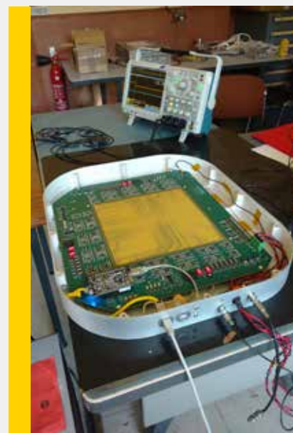
The current prototype with its 1600 channels: a compact system with the sensitive central area surrounded by the real time readout electronics
